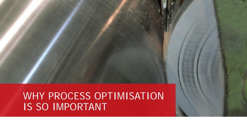
Material removal volumes of 0.05 to 3 mm are usual when grinding rollers. Depending on the type and size of roller, the grinding process can take between 15 to 50 minutes. As a result, the costs for the abrasive wheels make up the smallest proportion of the overall costs. As such, it is necessary to improve the added value potential by using an abrasive wheel that has been optimised for the application. This can substantially reduce the overall process costs:
