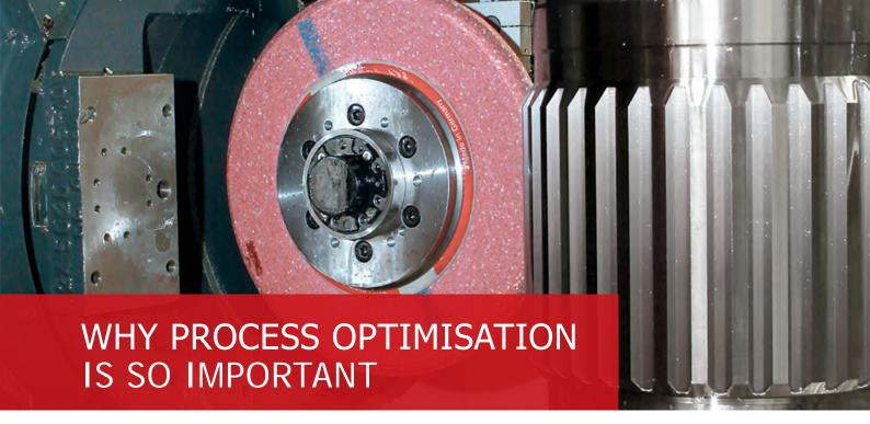
The "gear grinding" work process at the end of the process chain ultimately decides the quality of the gear wheel produced. Despite this, the cost of the abrasive wheel makes up only a small portion of the total costs. As such, it is necessary to improve the added value potential by using an abrasive wheel that has been optimised for the application. This can substantially reduce the overall process costs:
